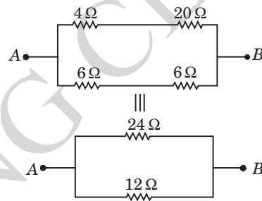
The equivalent resistance between  $A$  and  $B$  is
