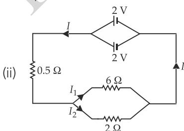
$$\text{Current in the circuit, } I = \frac{2 \text{ V}}{2 \Omega} = 1 \text{ A}$$
