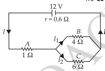
$$\text{Current in circuit, } I = \frac{12 \text{ V}}{4 \Omega} = 3 \text{ A}$$
