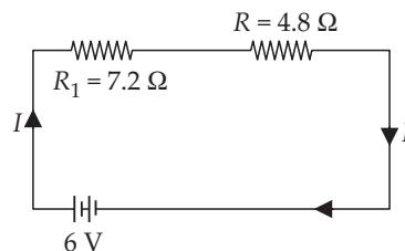
$R_1$  and  $R$  are in series, therefore total resistance of the circuit is
